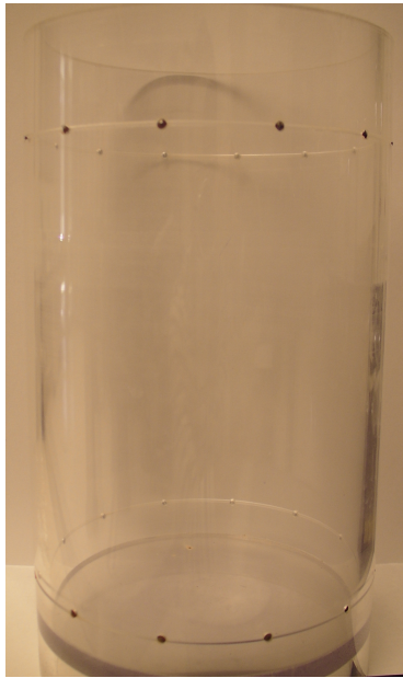
Figure 4.4: The PMMA cylinder (not filled with water), shown with the tracking beads for geometrical alignment corrections.
